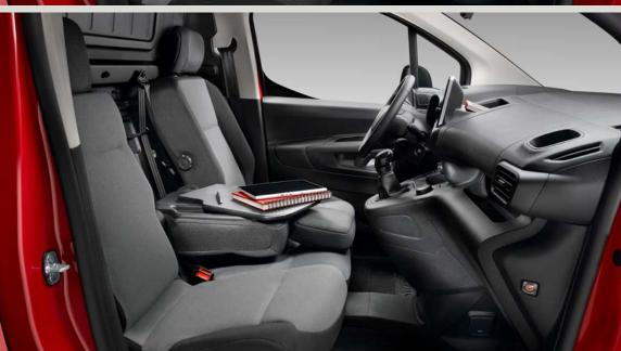
Fold the side passenger seat up to provide additional space for transporting fragile loads in the footwell.
