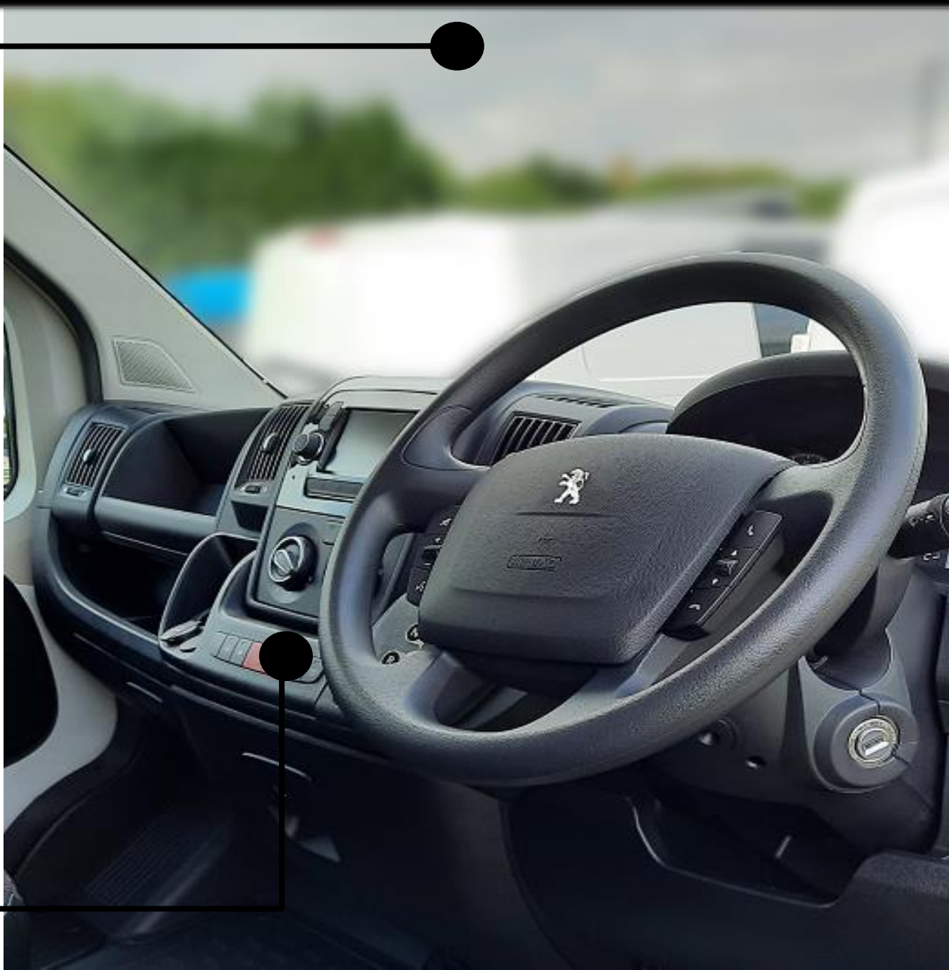
Gear Lever replaced with Drive Mode select buttons located to the left of the steering wheel
