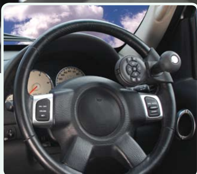
Remote control device incorporating steering wheel ball
